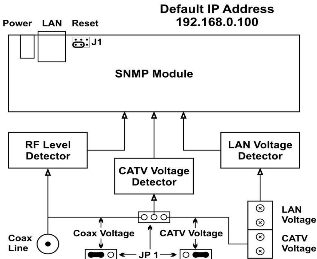
**Remote manage via SNMP v.1 protocol using built-in WEB interface.**
